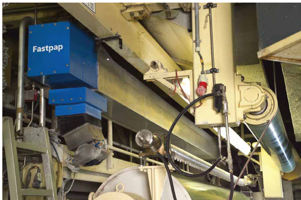
Fastpap LineSprint installed at a coating station for cleaning of the backing roll.
