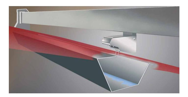
Fastpap ComboSprint is an efficient and reliable solution for cleaning the dryer fabric both during the process and web breaks. It cleans the fabric texture thoroughly without disturbing the moisture profile of the paper web.
